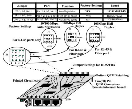
Figure 3.6 Combo ports, RJ-45 and Fiber internal jumper settings.
